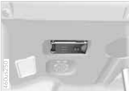
The interface socket for onboard diagnostics is located on the driver's side at the left-hand bottom of the dashboard and under a cover. The cover has the letters "OBD" on it.
