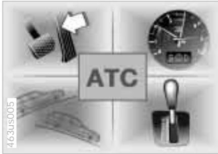
On vehicles with an automatic transmission, the Adaptive Transmission Control (ATC) uses a number of factors to calculate the gear which provides maximum efficiency. In this process, it considers your individual driving style as well as current driving conditions.
