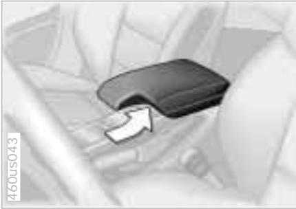
Open the storage compartment in the front center armrest\*: press the button (arrow) and lift upward.
