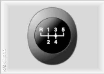
Completely depress the clutch pedal each time you shift, pressing the manual-shift gear lever into its respective end position.
