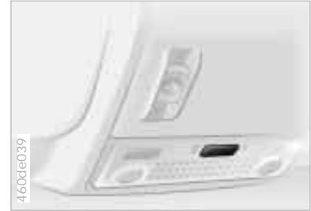
The illustration provides an example of the interior lamps when equipped with reading lamps.
