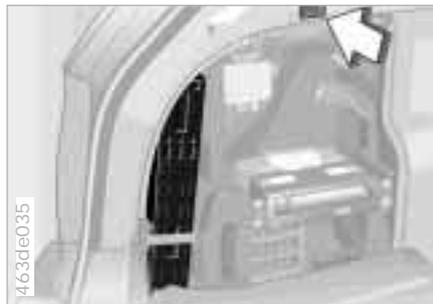
The hazard warning triangle is stored on the left-hand side of the luggage compartment behind the cover panel.
