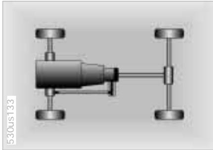
The transmission of power to the four drive wheels is provided permanently through a transfer box. The distribution of torque between the front and rear axles is 38 % to 62 %.
