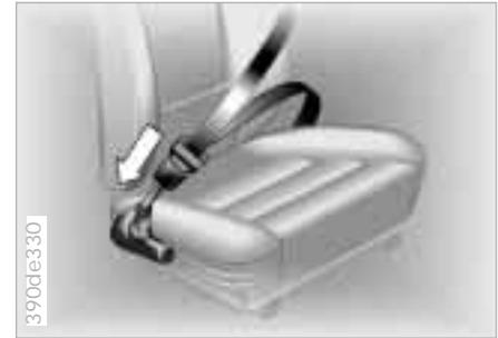
The safety belt tensioner responds to severe frontal collisions by tightening the belts to ensure that occupants remain firmly positioned in their seats. A gas-pressure system retracts the buckle assembly to tension the shoulder and lap belts within fractions of a second. This reduces the tendency to slide under the lap belt.
