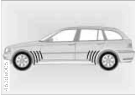
There is an antenna located right near every wheel in the vehicle body. This antenna picks up signals from its respective wheel. A central electronics system evaluates the quadruple signals which it receives and forwards any changes.
